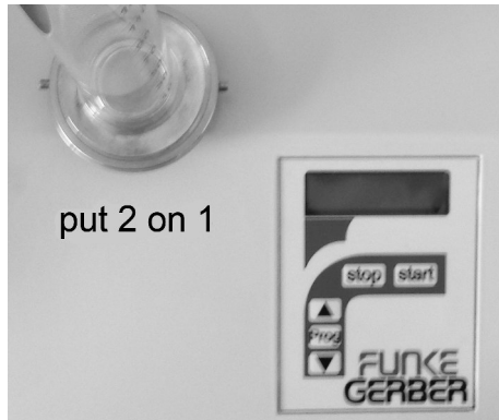
picture 4: installing measuring tank
