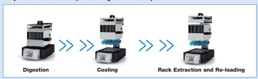
High performance and high reliability during sample preparation for Kjeldahl Analysis
