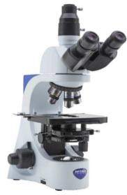
*Trinocular phase contrast microscope, 1000x, W-PLAN objectives*
