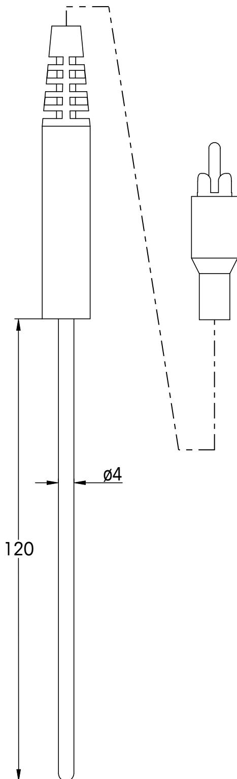
**Sensor type** temperature probe
