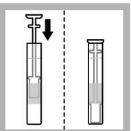
8. Add an optical tube insert to the second tube.
