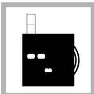
4. Put the tube into the left opening of the color comparator box.
