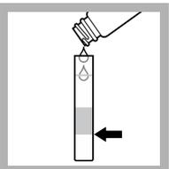
7. Fill a second tube to the first line (5 mL) with the prepared sample.
