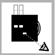
10. Read the value in the scale window. Divide the value by 5 to get the result in mg/L.
