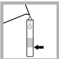
5. Fill a second tube to the first line (5 mL) with sample.
