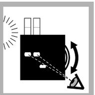
9. Hold the color comparator box in front of a light source. Turn the color disc to find the color match.
