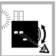
10. Hold the color comparator box in front of a light source. Turn the color disc to find the color match.
