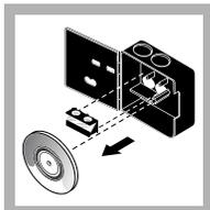
1. If installed, remove the long-path adapter.
