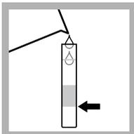
2. Fill a tube to the first line (5 mL) with sample.
