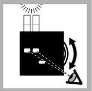
9. Hold the color comparator box below a light source. Turn the color disc to find the color match.
