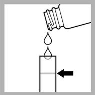
7. Fill a second tube to the top line with the prepared sample.
