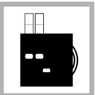
8. Put the second tube into the color comparator box.
