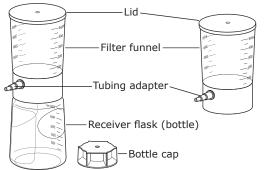
Stericup® and Steritop® systems come in different sizes to handle different sample capacities; the system components are the same except for capacity.
