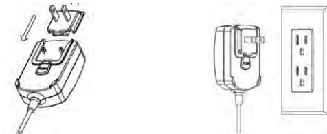
Figure 2-4. Connecting the AC adapter to AC supply
