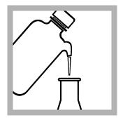
**6.** If the sample volume is less than 50 mL, dilute to approximately 50 mL with deionized water.
