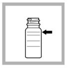
2. Blank Preparation: Fill one 25-mL mixing bottle with 25 mL of deionized water.
