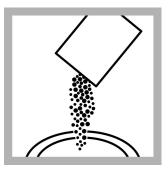
8. Prepare the sample: Use a funnel to add the contents of one NitraVer X Reagent B Powder Pillow to the vial.
