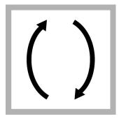
**9.** Close the vial. Invert the vial 10 times to mix. Some solid matter will not dissolve.
