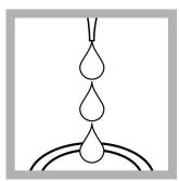
2. Prepare the blank: Use a pipet to add 1.00 mL of sample to a NitraVer X Reagent A Test 'N Tube vial.
