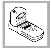
**14.** Install the instrument cap over the cell holder.
