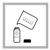
**2.** Prepare the sample: Fill a sample cell to the 10-mL mark with sample.
