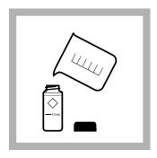
**5. Prepare the blank:** Fill a sample cell to the 10-mL mark with sample. Close the sample cell.
