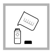
**6. Prepare the blank:** Fill a sample cell to the 10-mL mark with sample. Close the sample cell.
