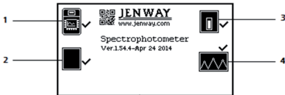
Fig 2.2.2 – All Power On Tests Complete
