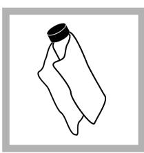
7. Use the oiling cloth provided to apply the oil equally to the surface of the sample cells. Remove the excess oil. Make sure that the sample cells are almost dry.
