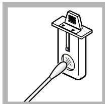
4. Clean the lens of the USEPA filter assembly. Refer to [Clean the filter assembly](#) on page 20.
