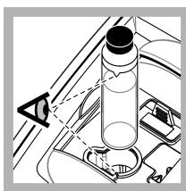
11. Put the vial in the sample cell holder with the triangle on the vial aligned with the reference mark on the sample cell holder. Push the lid closed until a click is heard.
