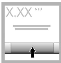
12. Push **Read**. Wait 1 minute for the instrument to complete the measurement.
