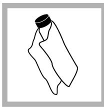
7. Get the StabCal standard that shows on the display. Clean the vial with a soft, lint-free cloth to remove water spots and fingerprints.
