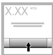
8. Push Read. The value and pass or fail status shows. The data is automatically stored in the instrument.
