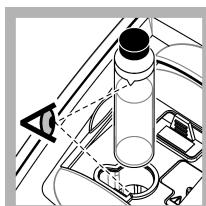
9. Put the sample cell in the sample cell holder with the triangle on the sample cell aligned with the reference mark on the sample cell holder. Push the lid closed until a click is heard.
