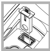
5. Hold the tab of the USEPA filter assembly so that the arrows point toward the front of the instrument. Push the filter assembly fully in the housing.
