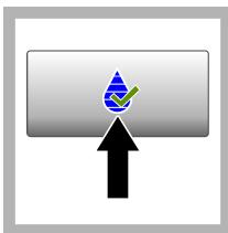
3. Push Verification. The verification standard value is shown. Push Options>Verification Setup to change the value of the verification standard.
