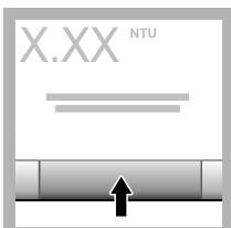
10. Push **Read** (or **Done** if in continuous mode). Wait for the instrument to read the sample.
