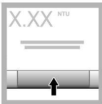
15. If Verify after Cal is set to on, the value of the verification standard shows. Push Read to measure the verification standard.
