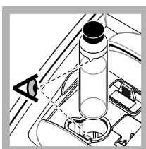
7. Put the vial in the sample cell holder with the triangle on the vial aligned with the reference mark on the sample cell holder. Push the lid closed until a click is heard.
