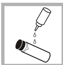
5. Apply a small drop of silicone oil from the top to the bottom of the vial.
