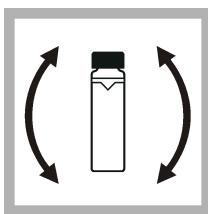
10. Carefully and slowly invert the vial to fully mix the standard (do not invert the <0.1 NTU vial). Be careful not to add air bubbles.
