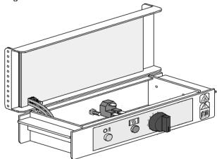
9.3.4. Remove any wire ties, now disconnect the heater leads from the amber neon.
