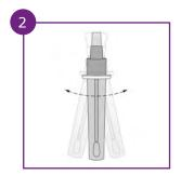
Place the swab into the extraction tube and carefully break off the end at the pre-scored point. Close the tube with a cap and shake vigorously for 1 minute.
