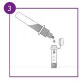
Remove the smaller cap to open the dropper tip and transfer **6 drops (200 \muL)** into an incubation vial. Close the lid of the vial.
