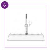
Place one test strip vertically (arrows pointing downwards) into the incubation vial. Incubate for 5 minutes. Read the result immediately.
