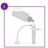
Add **0.2 mL** liquid sample (or rinse water), or weigh in **0.2 g** of homogenized sample into the extraction tube. Fill with **extraction buffer** to the level shown in the picture.
