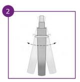
Close the tube with the cap and vigorously shake by hand for **1 minute**. You can squeeze the tube to help suspend the sample.
