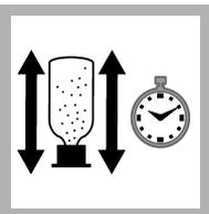
6. Keep the ampule inverted. Immediately put the cap on the tip of the ampule. Shake for 30 seconds.
