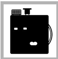
8. Put the ampule into the color comparator box.
