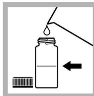
1. Fill a sample cell to the 10-mL line with the sample.
