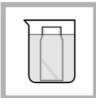
3. Collect 40 mL of sample in a beaker. Put the AccuVac Ampul Snapper in the beaker.
