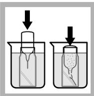
4. Invert one High Range Dissolved Oxygen AccuVac<sup>®</sup> Ampul. Put the ampule in the AccuVac Ampul Snapper. Push down to break and fill the ampule.
