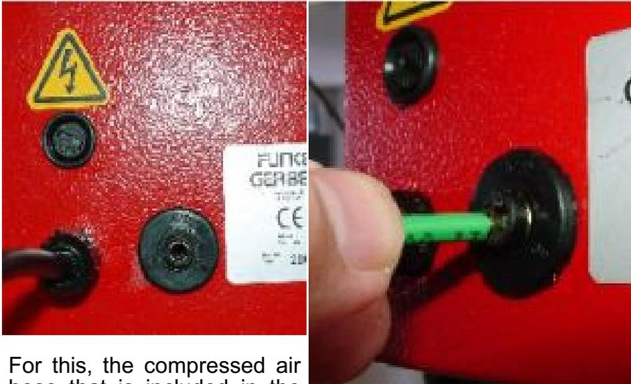
For this, the compressed air hose that is included in the scope of delivery is plugged into the compressed air outlet located on the back. The connection is airtight immediately upon connection.
