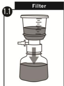
1.1 Filter: Filter sample through 0.45µm (micron) filter.
