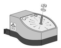
9.3.3. Turn the controller up-side down and remove the two fixing screws retaining the base. Lift the base off.
