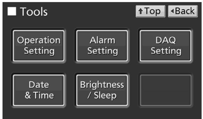
4. On the Date & Time screen, input the present date and time. Press Apply key to save the input value. The display returns to the Tools screen.
