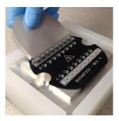
Tilt the tool backward so that the caps lift off.
