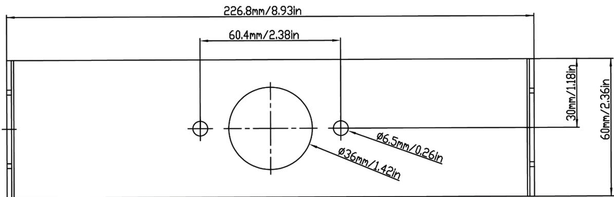
Figure 2-8 Dimensions du support de montage i-DT33XW
