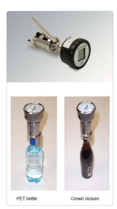
The Steinfurth Bottle Piercing Device is easily attached to glass bottles with crown closures or PET bottles. It pierces the closure, and the internal pressure can be read from the digital or analogue pressure gauge.
