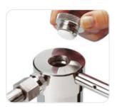
A practical filter holder for many laboratory filtrations. It can be attached to a tripod with the help of a steel rod which can be screwed in. The hose nipple is screwed into the side of the top part, leaving room for a large filling opening. This makes pouring in the sample easier, and the sample can be refilled without removing the tube connection to the pressure source. Leak-proof sealing is achieved by hand-tightening the
