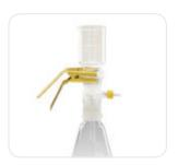
All areas, where liquid and device can come into direct contact, are made of glass or PTFE. The device, in combination with solvent-resistant, hydrophilic RC-membranes, is therefore ideal for ultracleaning and degassing solvents and solvent mixtures for HPLC, GC and AA. Convenience of handling is ensured by several beneficial features. A 6 mm wide non-ground rim
