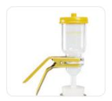
This filter holder is available in two versions differing from each other only in the type of the filter support. The device with glass frit ensures uniform distribution of retained particles and is therefore recommended, when the residue on the filter surface is of interest. Because it is easy to clean, the device with the PTFE-coated screen support is preferable when the filtrate is required, or when liquids difficult to remove from
