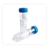
Vivaspin® Endotest is a disposable ultrafiltration device for endotoxin concentration and removal of substances interfering for the LAL test from liquid samples. The Vivaspin® Endotest is certified endotoxin free and available with a cellulose triacetate membrane of 20.000 MWCO. Due to the centrifugal design, Vivaspin® Endotest gives the opportunity to work in parallel which minimizes hands-on-time.
