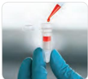
With the patented FlowGo regulator, the sample residence time is extended to assure adequate sample binding to the resin. As a result, Vivapure® Miniprep and Maxiprep spin column kits combine the merits of spin columns and gravity drip columns. This results in rapid purification with up to 95% protein recovery and purity.
