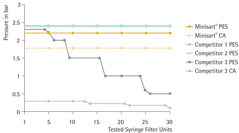
Method: Pressure-hold tests were performed by connecting pre-wetted syringe filter units to a 10-fold pressure device with a pressure gauge. The pressure applied equaled 4/5 of the bubble point. Units failed the test if they released air bubbles before reaching 4/5 of the minimum bubble point. These units were remeasured to determine at which pressure air bubbles appear.
