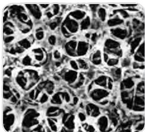
Cellulose acetate membranes combine high flow rates and thermal stability with very low adsorption characteristics, and are therefore excellently suited for use in pressure filtration devices. They are hydrophilic, have high flow rates thanks to their symmetric structure and are compatible with aqueous solutions
