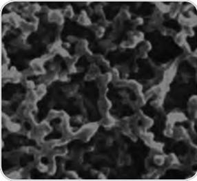
Polyamide membrane filters are hydrophilic and chemically resistant to alkaline solutions and organic solvents. They are therefore recommended for the particle removal from aqueous solutions and
