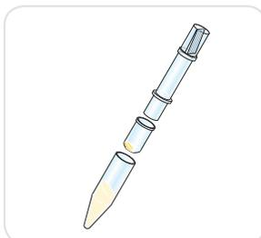
Direct pipette recovery or choice of reverse spinning concentrate into sample cap
