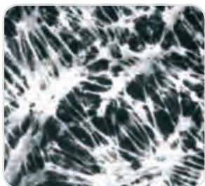
The main application of these membrane filters is the filtration of air, gases or chemicals. They are made of PTFE (polytetra-fluoroethylene) only and are therefore permanently hydrophobic. Unlike other (hydrophilic) filter types, they are not wetted by air humidity, allowing unhindered passage of air at low differential pressures as well. PTFE
