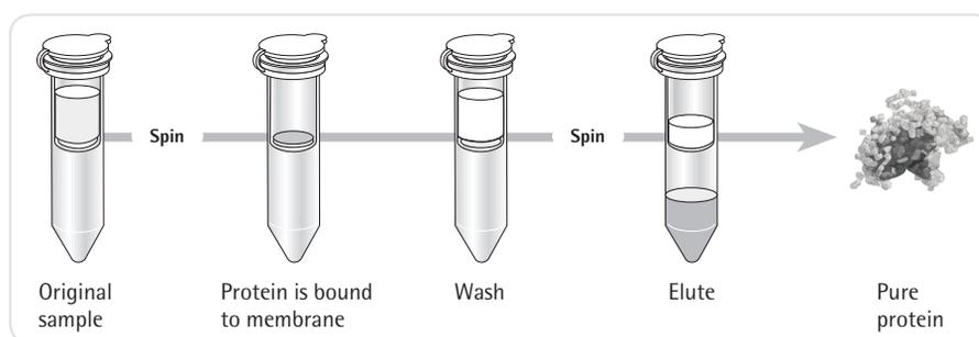
Fast and easy protein purification with Vivapure<sup>®</sup> spin columns
