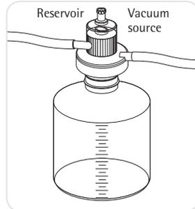
Place Sartolab® 150v on the bottle neck. Vacuum is automatically created when used with a water jet pump or a different vacuum source.
