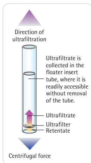
Centrisart® I\* is a ready-to-use unit for small-volume, centrifugal ultrafiltration to separate proteins from low molecular weight substances in biological samples.
