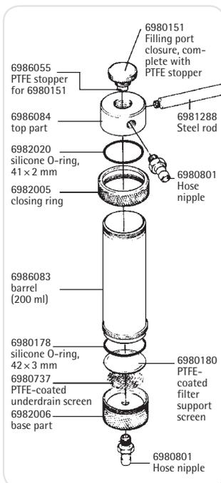
A practical filter holder for many laboratory filtrations. It can be attached to a tripod with the help of a steel rod which can be screwed in. The hose nipple is screwed into the side of the top part, leaving room for a large filling opening. This makes pouring in the sample easier, and the sample can be refilled without removing the tube connection to the pressure source. Leak-proof sealing is achieved by
