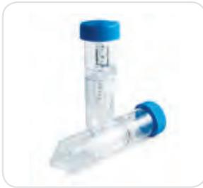
Vivaspin® Endotest is a single-use ultrafiltration device for endotoxin concentration and removal of interfering substances from liquid samples for LAL testing. The Vivaspin® Endotest is certified as endotoxin-free and is available with a cellulose triacetate membrane that has a molecular weight cutoff (MWCO) of 20,000.
