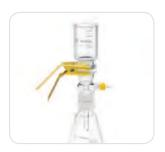
All areas, where liquid and device can come into direct contact, are made of glass or PTFE. The device, in combination with solvent-resistant, hydrophilic RC-membranes, is therefore ideal for ultracleaning and degassing solvents and solvent mixtures for HPLC, GC and AA. Convenience of handling is ensured by several beneficial features. A 6 mm wide
