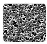
Polyethersulfone (PES) membrane filters are hydrophilic, have high flow rates thanks to their symmetric structure, have a low non-specific protein adsorption and are chemically resistant over a pH range of
