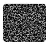
Cellulose nitrate membrane filters are indicated for many general laboratory applications where a membrane with a high non-specific adsorption is suitable. They are hydrophilic, have high flow rates thanks to their symmetric structure and are compatible with aqueous solutions
