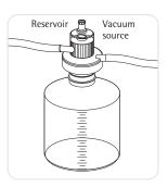
Place Sartolab® 150v on the bottle neck. Vacuum is automatically created when used with a water jet pump or a different vacuum source.
