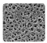
The very low adsorption membranes are hydrophilic, solvent-resistant (pH 3-12) and therefore suited for the particle removal from solvents. The membrane is asymmetric
