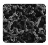
Polyamide membrane filters are hydrophilic and chemically resistant to alkaline solutions and organic solvents. They are therefore recommended for the particle removal from aqueous solutions and
