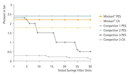
Method: Pressure-hold tests were performed by connecting pre-wetted syringe filter units to a 10-fold pressure device with a pressure gauge. The pressure applied equaled 4/5 of the bubble point. Units failed the test if they released air bubbles before reaching 4/5 of the minimum bubble point. These units were remeasured to determine at which pressure air bubbles appear.
