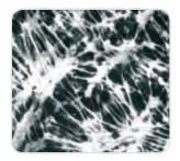
The main application of these membrane filters is the filtration of air, gases or chemicals. They are made of PTFE (polytetra-fluorethylene) only and are therefore permanently hydrophobic. Unlike other (hydrophilic) filter types, they are not wetted by air humidity, allowing unhindered passage of air at low differential pressures as well. PTFE
