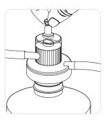
To fill multiple receiving bottles, break the vacuum by opening the valve on top of the Sartolab® 150v housing.
