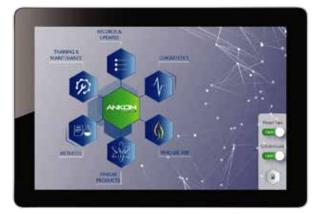
The ANKOM<sup>*FLEX*</sup> Analyte Extractor has touch screen functionality and a user-friendly interface powered by state-of-the-art software. Digestion time, temperature, and pressure is monitored and controlled at all times. The user has a complete history of their research and instrument performance, which can be exported to other platforms.
