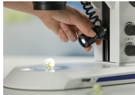
Change height of the spot and zoom in to create distinct shadows for a strong 3D impression. In the lowest position it delivers a grazing light that enhances fine structures on flat surfaces via hard shadows.
