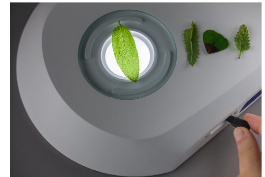
Use the flat transmitted light unit to contrast colored transparent specimens in bright- and darkfield. Add polarizer/analyzer equipment to observe, for example, birefringent crystals or tensions in glass or plastics.
