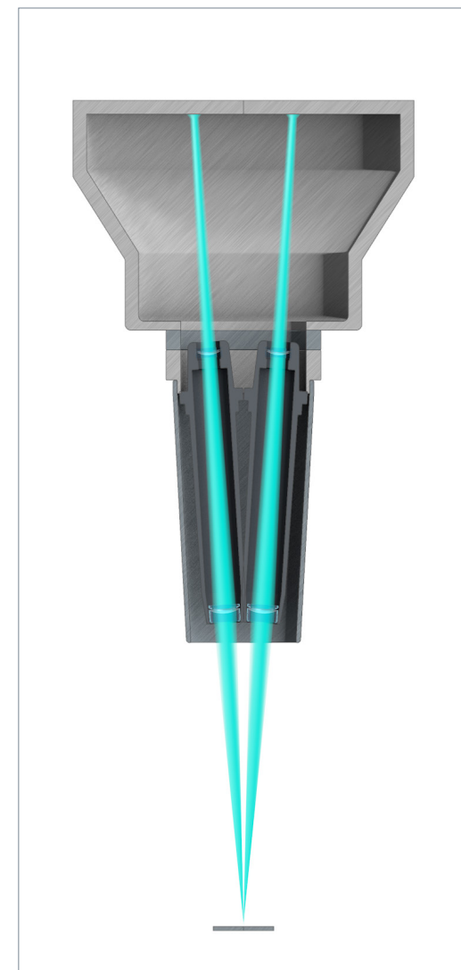
Beam path of a Greenough type stereo microscope
