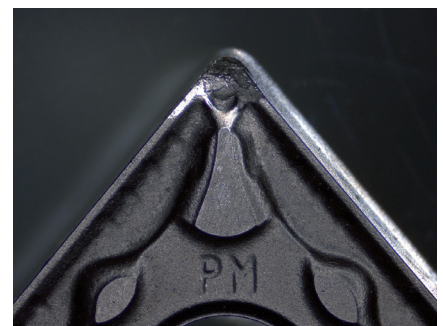
Indexable insert, shows tool wear. Reflected light, ringlight, zoom 0.8x
